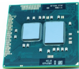
Intel Core i5 processor Real size: 3.75cm x 3.75cm
