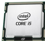
Intel Core i5 processor Real size: 3.75cm x 3.75cm
